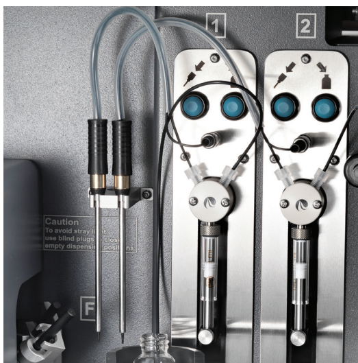
Figure 1. Reagent dispensers allow for easy and accurate reagent addition.
